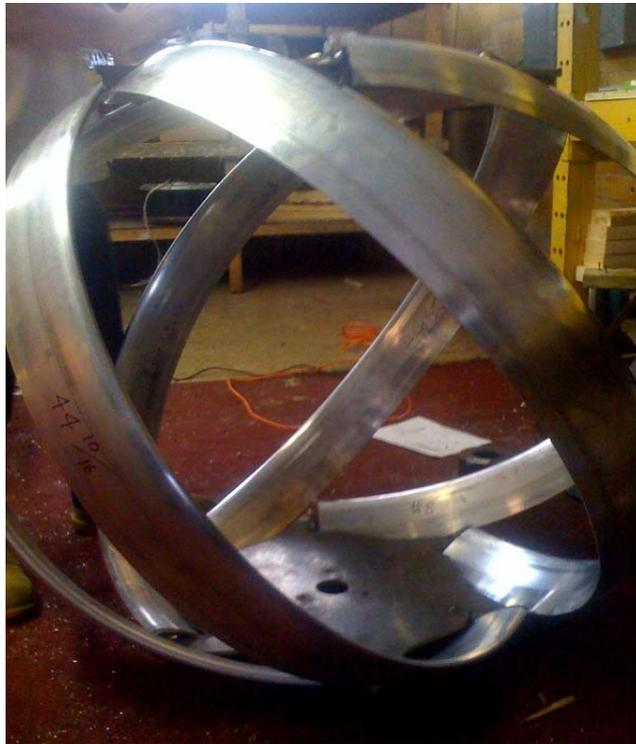
**Figure 9. Lucid Spherical Turbine as tested**
