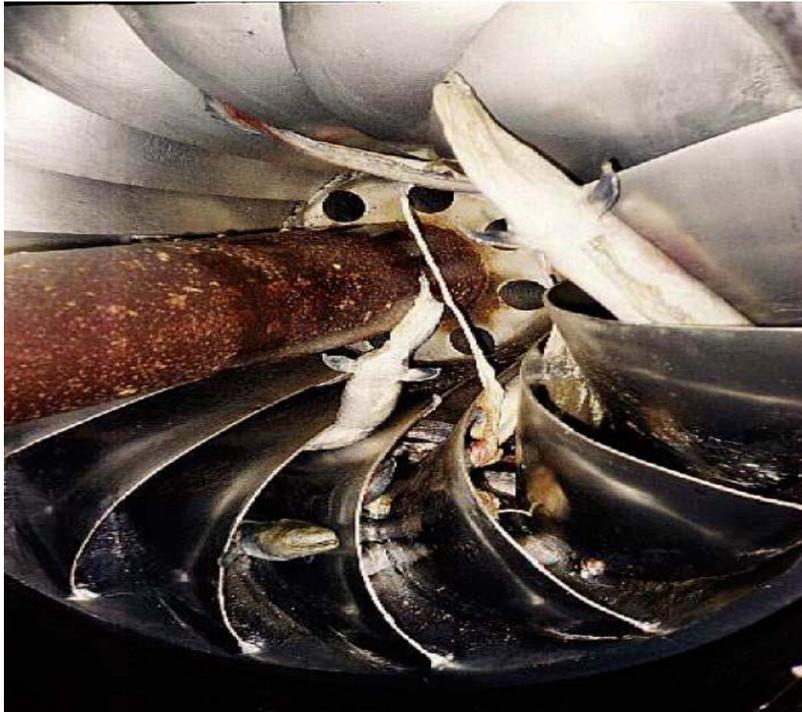
**Figure 3. Turbine clogged with eels. Note eel skin stretched across shaft.
