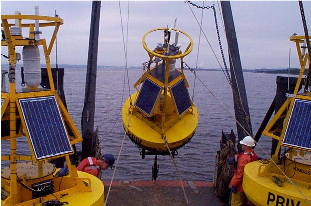
Figure 6. GoMOOS buoy J02 being retrieved for servicing by U. Maine, Orono staff aboard the R/V Argo Maine. The meteorological sensors are on top of the tower. The sensor just below the buoy is the Aanderaa current meter at 2 m depth. The GoMOOS buoys are serviced at 6-month intervals, or when repair is needed. Newly refurbished buoys are seen on either side of the deck, ready for deployment.
