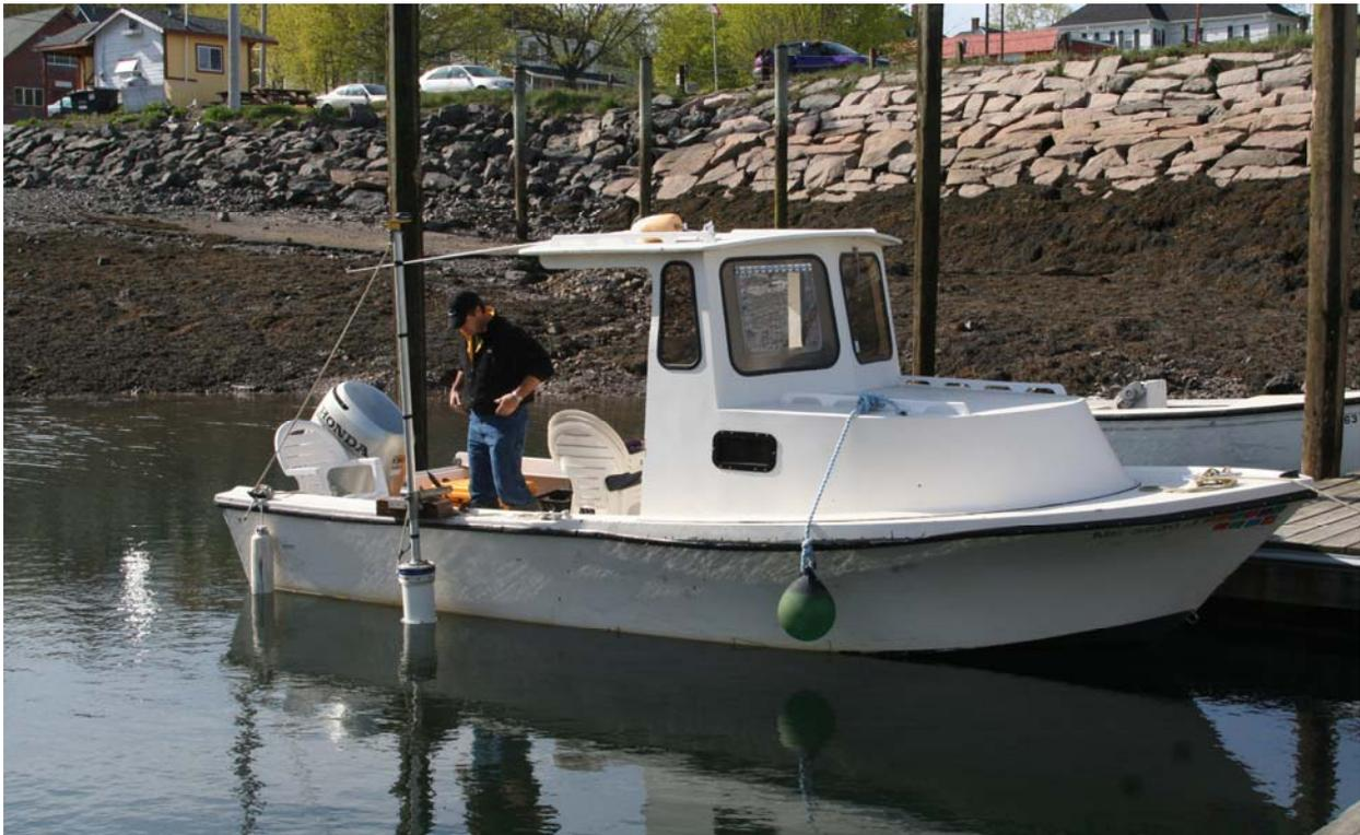
*Figure 1. The RD Instruments ADCP mounted on the side of the survey vessel in Eastport Harbor, ME. The GPS receiver is located on top of the pole holding the ADCP. Pete Feeney is seen on deck. The computer logging was done in the ship's cabin.*
