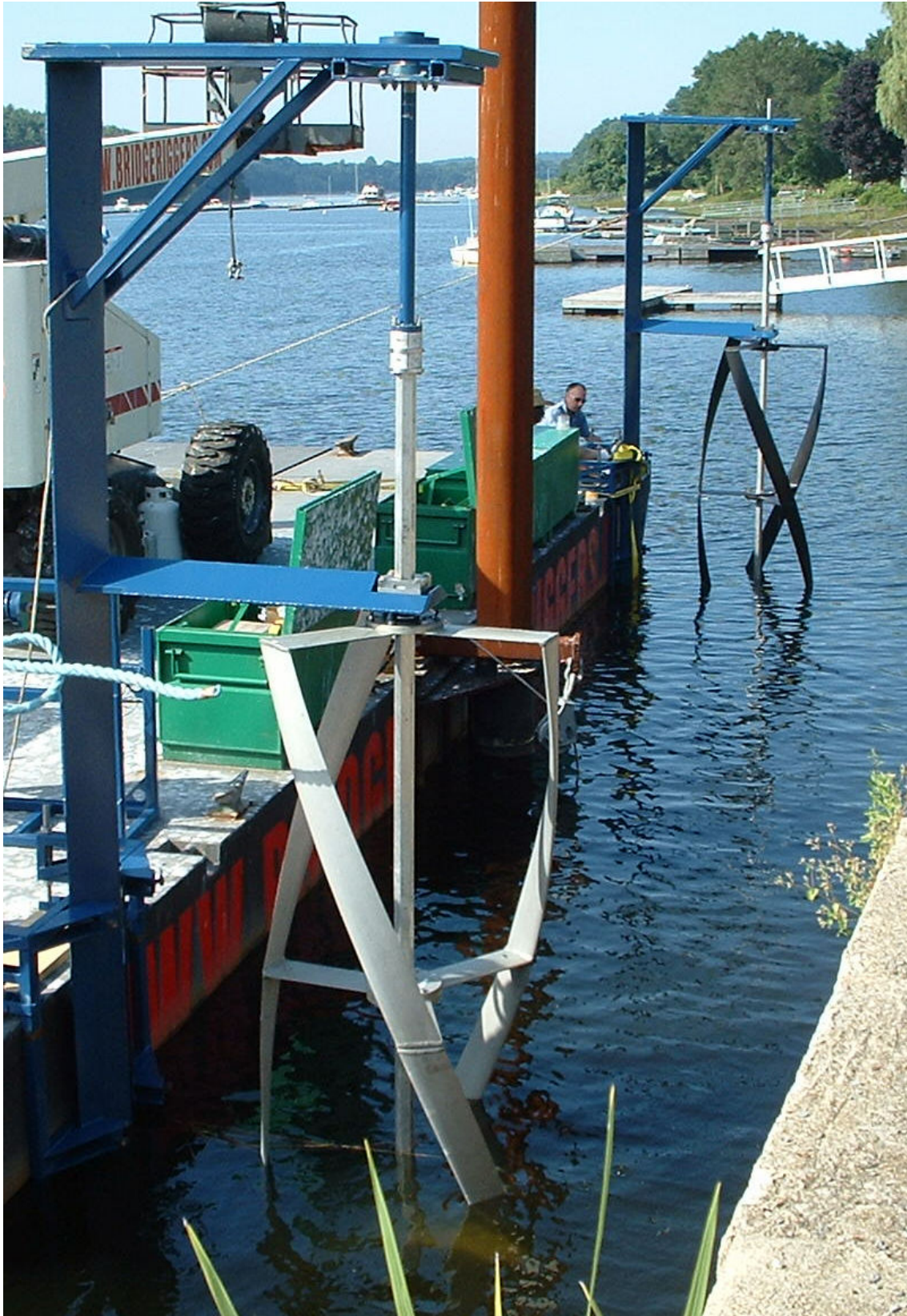
Figure 2 GHT Rotors #1 and #2 Mounted in VP Frames ( patents pending ) for Testing
