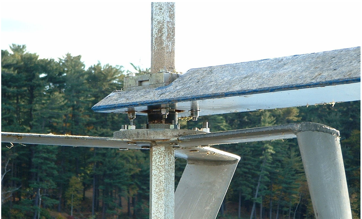
Figure 37. Minor Surface Fouling On Rotor and Frame
